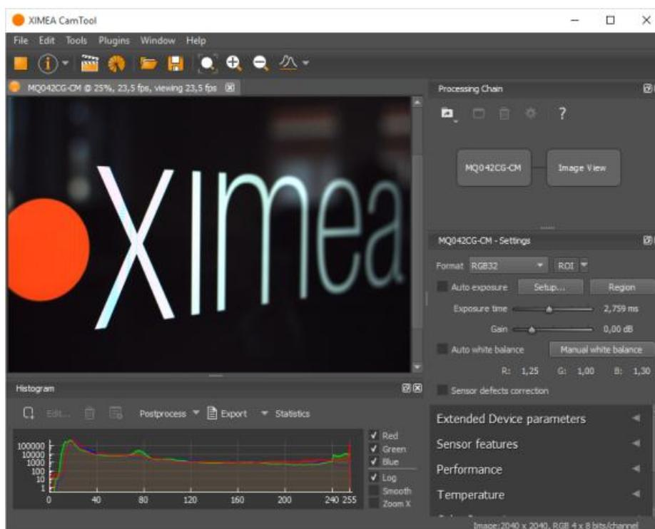
CamTool supports the Processing chain feature (top right in the picture) where the user can see the pipeline of processes from the camera to view, and split it into multiple views.
